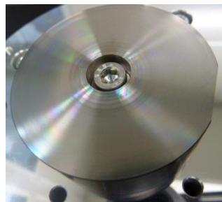
aerostat. Spindel; v = 80\text{m/min} , f = 4,8\text{ mm/min} , a = 10\text{ }\mu\text{m}
